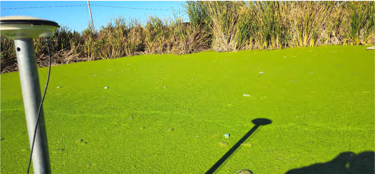
Digital Image 5. Tobermory East Secondary Cell 2. Conducting baseline sludge sub-bottom/liner and bathymetry, sludge blanket depths for post-processing validation.
