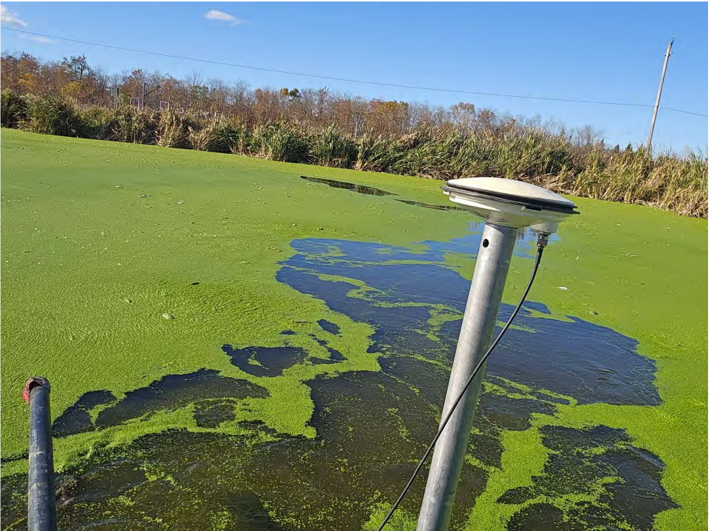
Digital Image 4. Tobermory East Secondary Cell 2. Conducting baseline sludge sub-bottom/liner and bathymetry, sludge blanket depths for post-processing validation.
